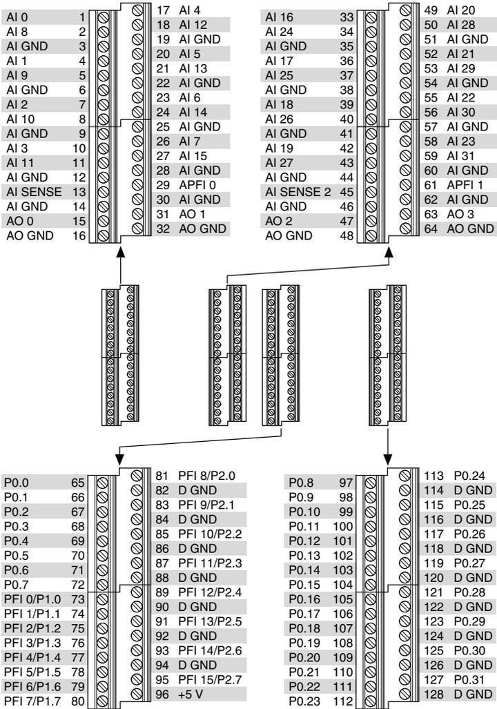
**Figure 12. NI USB-6259 Mass Termination Pinout**
