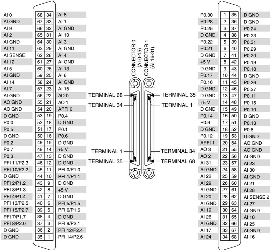
**Figure 10. NI USB-6259 Screw Terminal Pinout**
