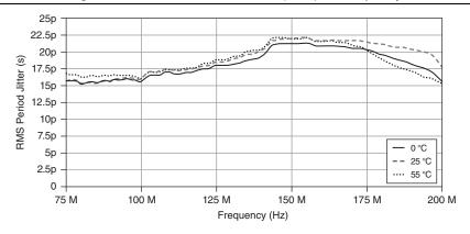
Figure 1. Characteristic Period Jitter (RMS) vs. Frequency
