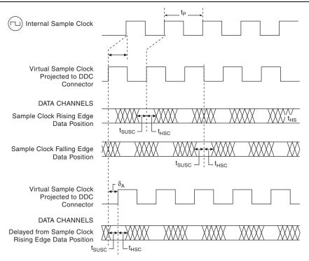
t<sub>DDCSC</sub> : Time Delay from DDC Connector to Internal Sample Clock
