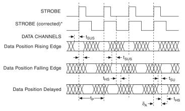
t<sub>SUS</sub> = Set-Up Time to STROBE
