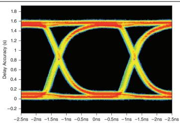
Figure 3. Characteristic Eye Diagram (50  $\Omega$  Termination)
