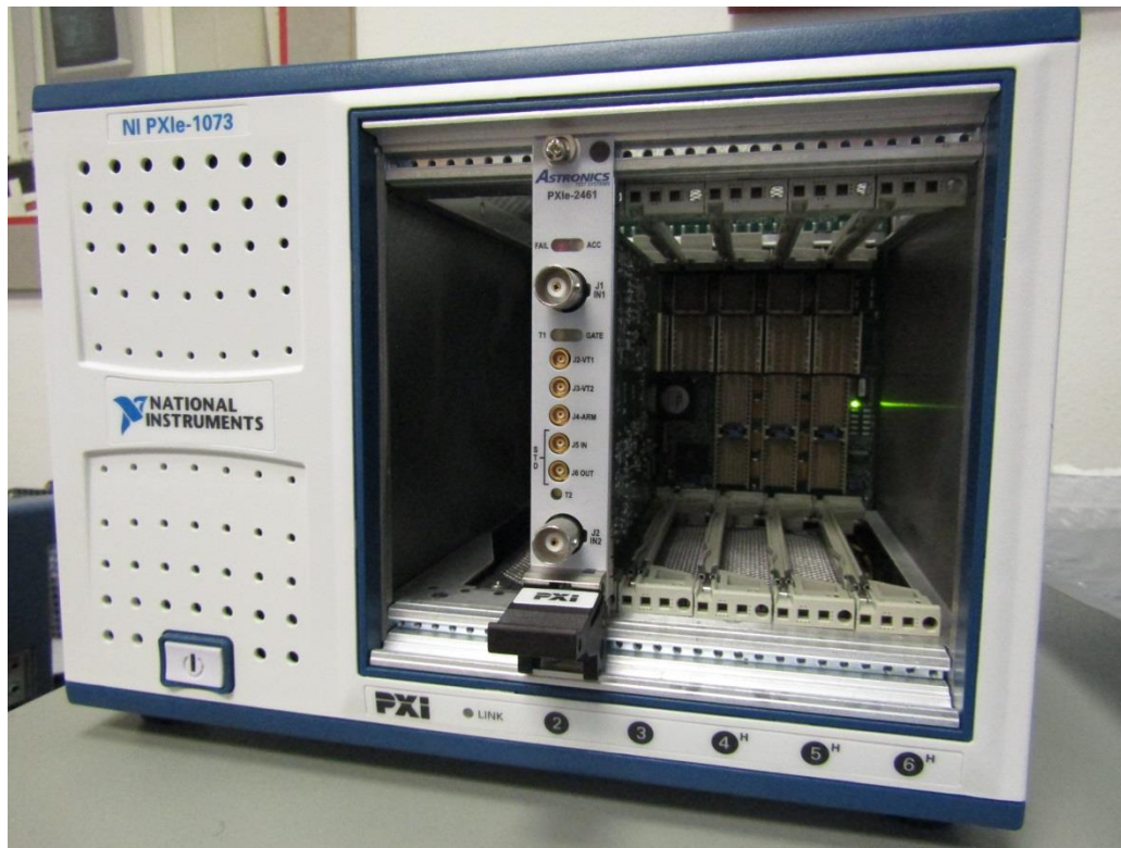
Figure 2-1 PXle-2461 Chassis Installation
