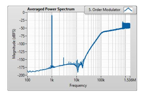
\* Measurement Conditions: PDM rate = 3.072 MHz; Modulator bandwidth = 20 kHz; Test frequency = 1 kHz; Test amplitude = 0.5 FS; Spectral resolution = 10 Hz; Window type = Hanning; Number of RMS averaging = 64.
