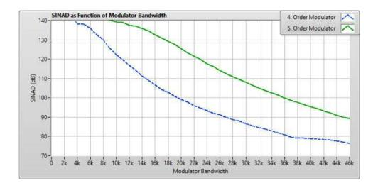
\* Measurement Conditions: PDM rate = 3.072 MHz; Modulator bandwidth = 3 kHz to 46 kHz; Test frequency = 1 kHz; Test amplitude = 0.5 FS.
