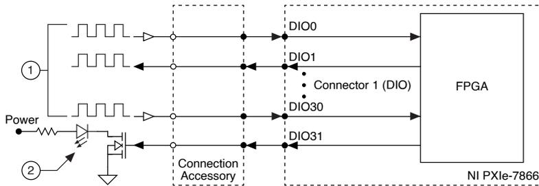
1. High-speed signal frequencies up to 20 MHz that is compatible with 5 V TTL, 3.3 V LVTTTL, and 3.3 V LVCMOS.
