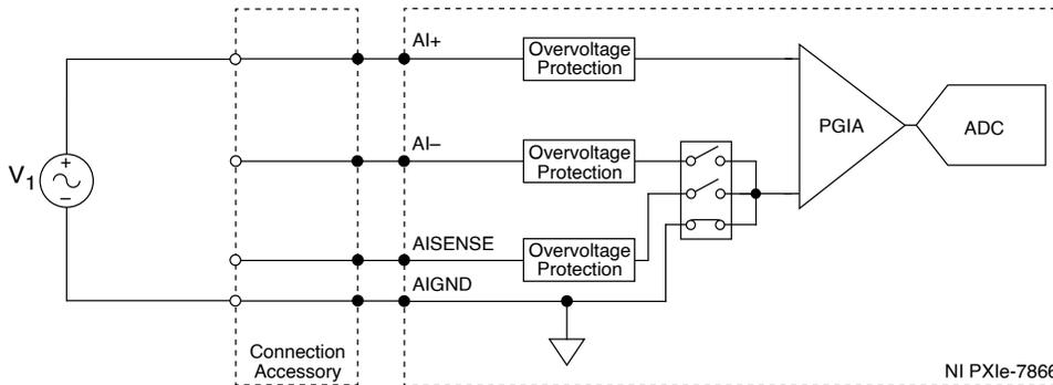
To connect non-referenced single-ended voltage signals to the NI PXIe-7866, you must connect the voltage ground signal to AI SENSE in order to keep the common-mode voltage in the specified range.
