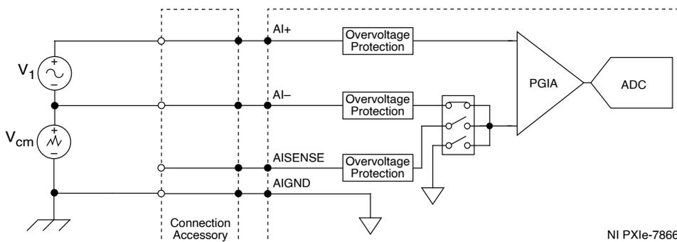
To connect floating differential signals to the NI PXIe-7866, you must connect the negative and positive signals to AI GND through 1 M $\Omega$  resistors to keep the voltage within the common-mode voltage range. If the voltage source is outside the common-mode voltage range, the NI PXIe-7866 does not read data accurately.
