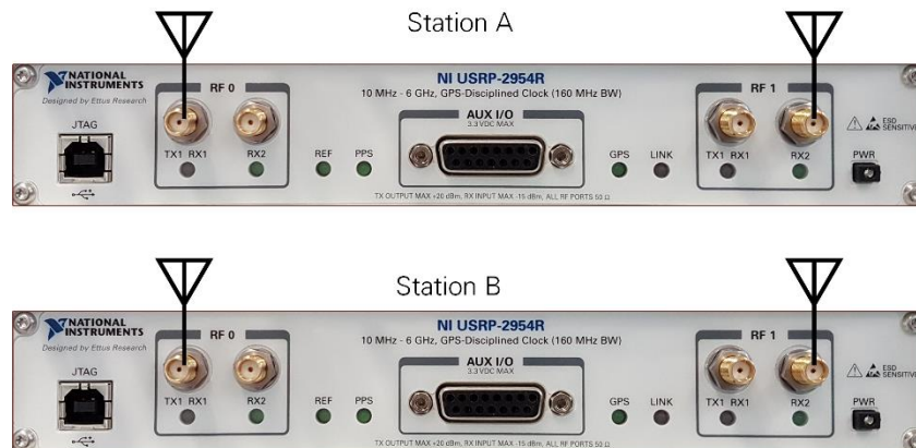
Figure 4 Antenna Connection for USRP Devices
