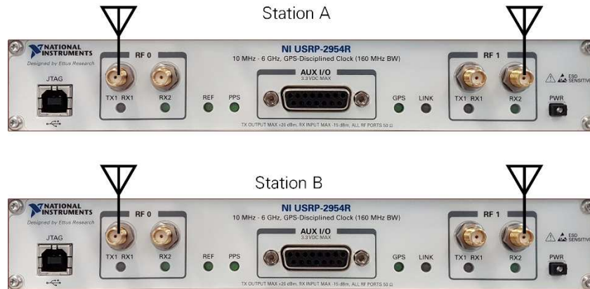
Figure 3 Antenna Connection for USRP Devices
