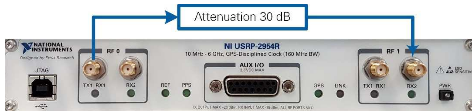
Figure 10 USRP Hardware Configuration
