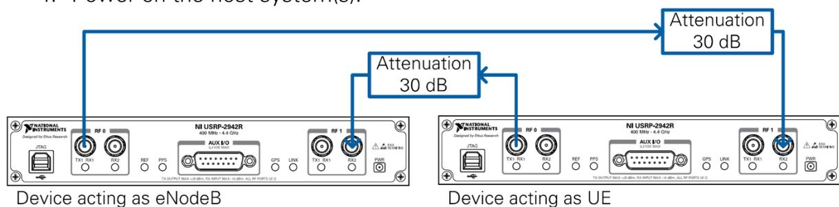
Figure 12 Cabled Connection of Two USRP Devices
