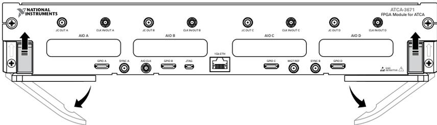
2. Gently guide the module into the chassis module guides and slide the module into the chassis until it is fully inserted.
