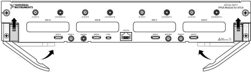
4. Tighten the four captive screws on the panel to secure the module.
