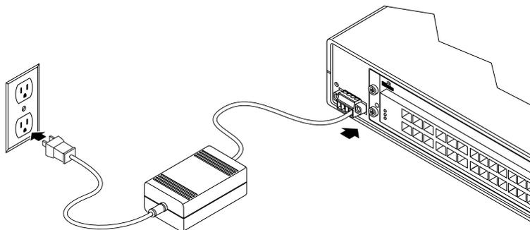
The ATCA-3671 powers on automatically once the DC power supply is connected to the power source.
