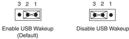
Figure B-3. Enable/Disable USB Wakeup Jumper: JPUSB1
