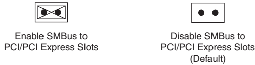
Figure B-7. Enable/Disable SMBus to PCI/PCI Express Slots Jumper: JI 2 C1/JI 2 C2
