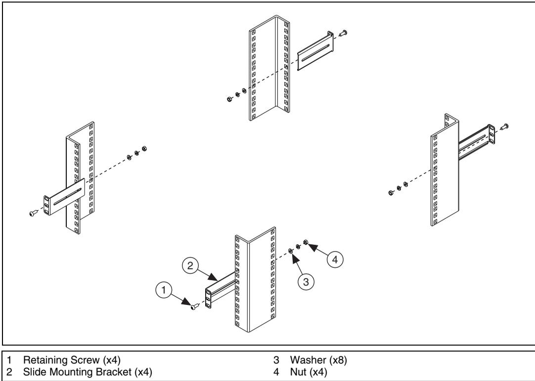
**Figure 2-3.** Installing Slide Mounting Brackets in Rack
