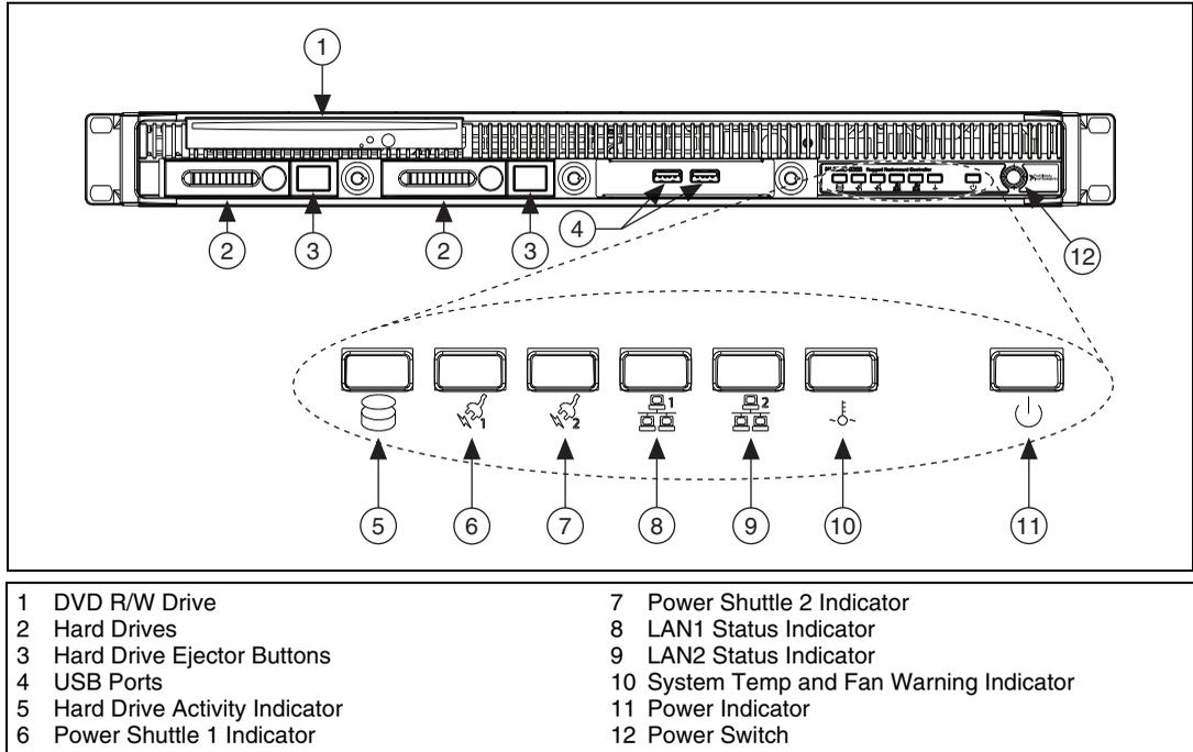
**Figure 1-1.** Front View of the NI RMC-8355
