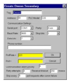
**Serial port** specifies which comm port the object uses for communicating to the external device. This does not specify the communication type. Communication type is determined by the Options—Serial Ports... command.
