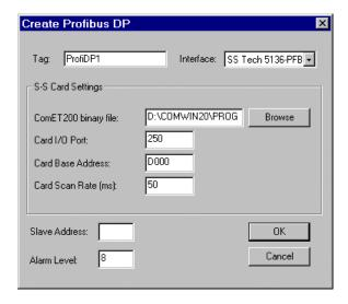
**Interface** is the type of card to be used to communicate with the DP network. At present, this driver only supports the S-S card interface.
