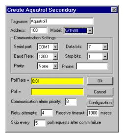
**Address** is the address of the RTU as configured on the device. The address can be in the range of 100 to 999 inclusive.
