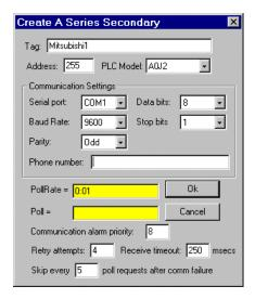
**Serial port** specifies which comm port the object uses for communicating to the external device. This does not specify the communication type. Communication type is determined by the <a href="Options-Serial Ports...command">Options-Serial Ports...command</a>.
