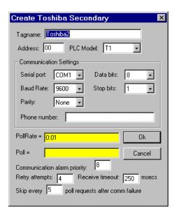
**Address** specifies the address of the PLC. The maximum address for a T Series PLC is 32 and for an M Series PLC, 15.
