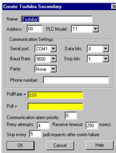
**Figure 3-42.** Toshiba T Series Configuration Parameters Dialog Box
