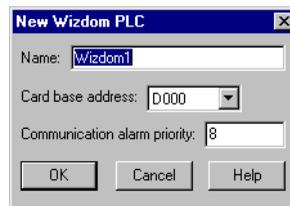
**Card base address** specifies the beginning memory location of the dual ported RAM address. It should match jumper settings on the card. The card uses 8K of physical memory.
