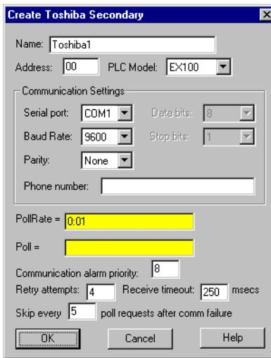
**Figure 3-41.** Toshiba M Series Configuration Parameters Dialog Box
