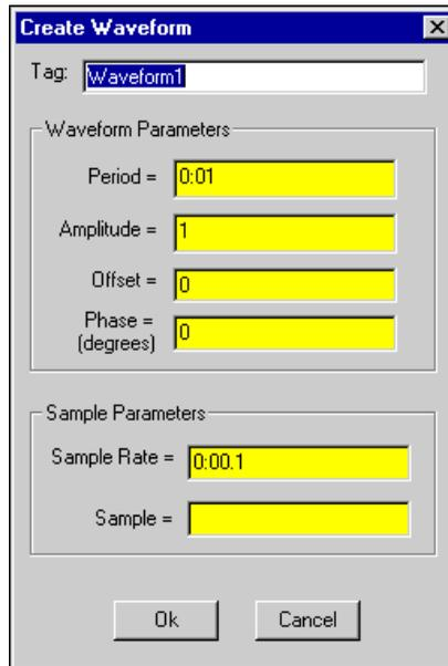
The Waveform object produces output by sampling the desired waveform at the specified **Sample Rate**. The **Period** (in days), **Amplitude**, **Offset** (level shift), and **Phase** (in degrees) of the generated waveforms can be set to any numerical expression. A single Waveform object can be used to generate multiple waveforms of varying relative phases, all with the same **Period**, **Amplitude**, **Offset** and absolute **Phase**.
