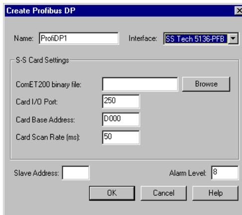
**Figure 3-32.** Profibus DP Configuration Parameters Dialog Box
