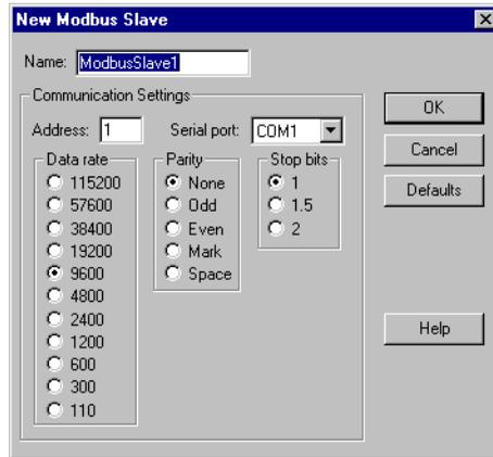
**Figure 3-20.** Modbus Slave Configuration Parameters Dialog Box
