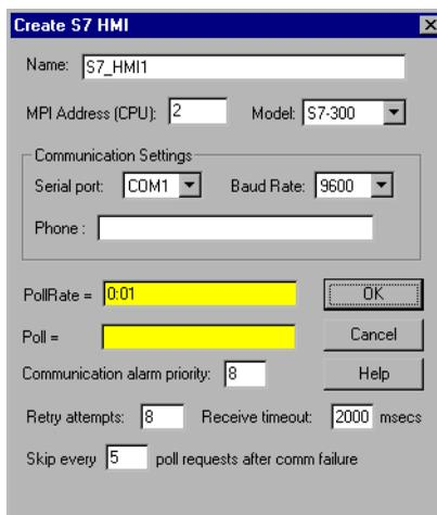
**Serial port** specifies the COM port on the host computer that Lookout object uses for communicating to the external device. This does not specify the communication type. Communication type is determined by the **Options»Serial Ports** command. See Chapter 3, *Serial Port Communication Service*, of the *Lookout Developer's Manual* for more information on configuring your serial ports for use with Lookout.
