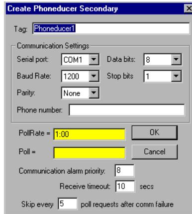
**Serial port** specifies which COM port on the host computer that Lookout object uses for connecting to the modem used to dial up the Phoneducer. See Chapter 3, *Serial Port Communication Service*, of the *Lookout Developer's Manual* for more information on configuring serial ports for use with Lookout.
