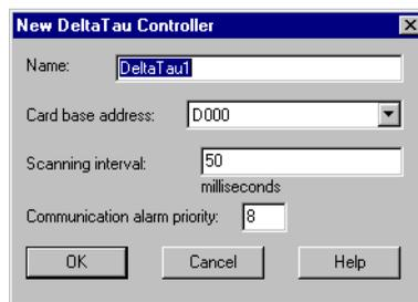
**Card base address** specifies the beginning memory location of the dual ported RAM address. It should match card settings.
