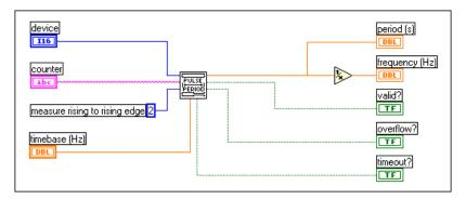
Figure 26-9. Diagram of Measure Period-Easy (DAQ-STC) VI
