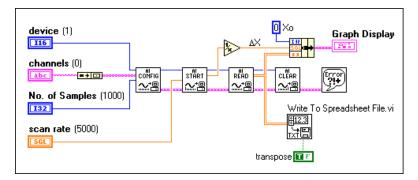
**Figure 7-8.** Writing to a Spreadsheet File after Acquisition
