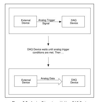
Figure 8-5. Analog Triggering with Your DAQ Device
