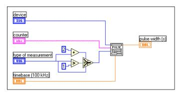
Figure 25-3. Diagram of Measure Pulse Width (DAQ-STC) VI
