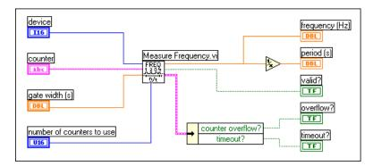
Figure 26-6. Diagram of Measure Frequency-Easy (9513) VI
