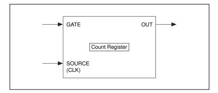
A counter consists of a SOURCE or CLK input pin, a GATE input pin, an OUT output pin, and a count register. In plug-in device diagrams and in the LabVIEW Function Reference and VI Reference Manual, these counter parts are called SOURCEn (or CLKn), GATEn, and OUTn, where n is the number of the counter.
