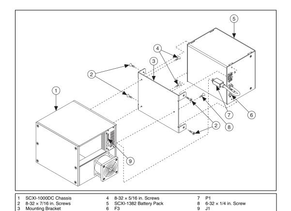
Figure 1. Connecting the SCXI-1382 to the SCXI-1000DC Chassis
