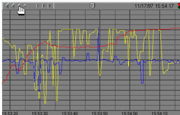
The button bar includes scroll arrows, a cursor button, date, time, and a stop & go light. Use the **scroll arrows** to move back and forth through time—the bigger the arrow button you select, the further the trend jumps in time. The scroll arrows also function much like a horizontal slider. Click on them and slide the mouse left and right while holding down the mouse button. The further you slide the cursor from dead center, the faster the trend scrolls in that direction.
