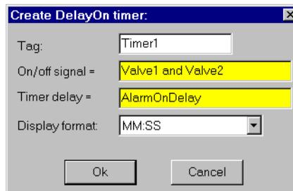
The parameter **On/off signal** expects a logical expression and **Timer delay** requires a numeric expression. Both `Valve1` and `Valve2` are tagnames for switches. Connecting them with *and* produces a logical result and satisfies the type condition of the first parameter. `AlarmOnDelay` is the tagname of a potentiometer used to adjust the timer delay setpoint, which creates a numeric signal, satisfying the type condition of the second parameter.
