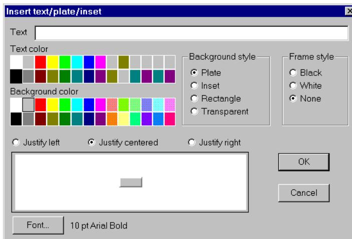
If you want to create a rectangle, line, plate or inset, leave the **Text** field blank and choose a **Background style**. The preview window displays the element as it appears on a control panel.
