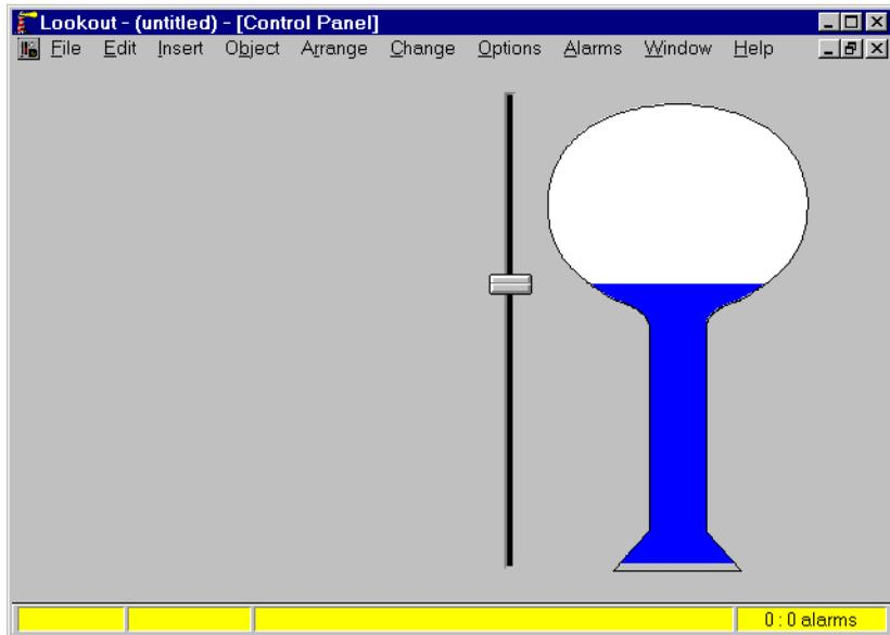
Press <CTRL-SPACE> to toggle out of edit mode and move the slider up and down to see the fill effect created with your tank mask and bar graph. Then get back into edit mode so you can create a trend of the tank level.
