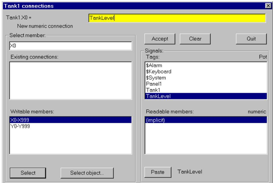
The Interpolate object now multiplies the X0 input by the **Input(x) multiplier**, find the two coordinate pair parameters that X0 falls between, interpolate, and multiply the interim output by the **Output(y) multiplier**, then send the resulting value to the Y0 readable data member.
