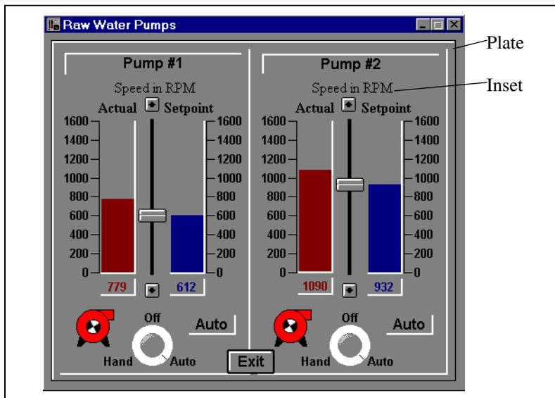
To create static text, plates, insets, rectangles or lines in Lookout, select the **Insert>Text/plate/inset...** command. The following dialog box appears.
