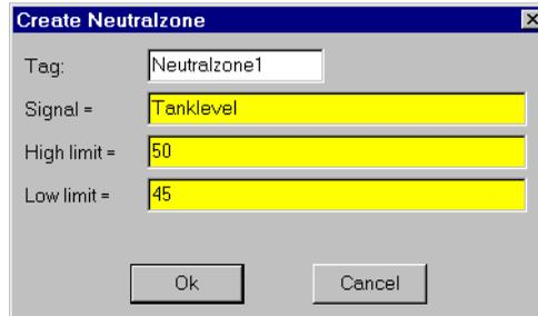
Avoid using the *is equal to* (=) and *is not equal to* (<>) comparison operators to compare an analog value from a PLC or the result of mathematical calculations in an expression. Because numeric (floating point) values have about 17 significant digits, `TankLevel = 40` might never be exactly true. If you know the signals are integer values, such as the numeric signal from the potentiometer in the following example, use the = and <> operators.
