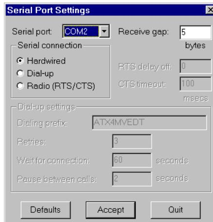
Now connect a Modbus protocol controller to your process. First you must create a Modbus object with **Object»Create....**
