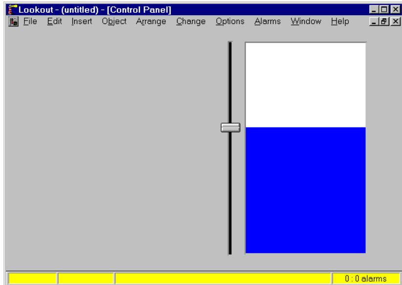
This bar graph simulates the water level in the tank. To give it a more realistic look, lay a graphic of a tank on top of it to act as a mask.
