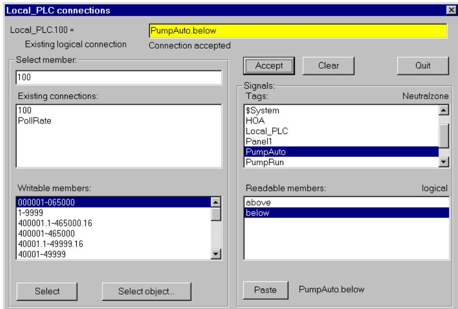
You now need to create another Modbus object for the remote RTU. Each controller has its own respective object in Lookout. Each of these objects determines its polling scheme, read/write blocking, and so on.
