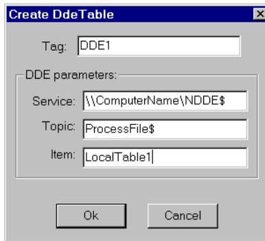
**Figure 18-31.** DdeTable Definition Parameters Dialog Box (Remote Computer)
