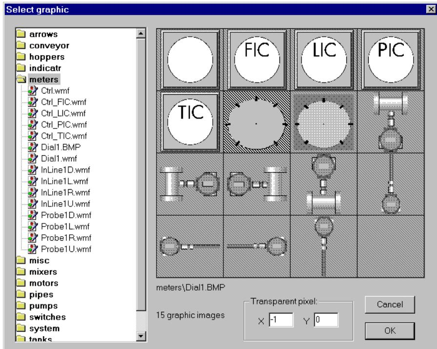
You can use a multicolor bitmap as a type of mask. For this to work, inside of the bitmap (the gray area) must be transparent and the rest of the graphic opaque—masking the underlying part of the control panel. You can insert another Lookout element, such as a bar graph, to furnish a convenient visual warning, such as a rising color level.
