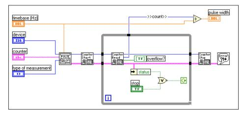
Figure 25-8. Measuring Pulse Width with Intermediate VIs
