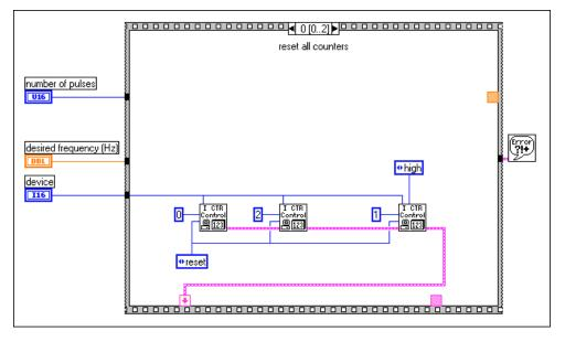
Figure 24-25. Frame 2 of Finite Pulse Train (8253) VI
