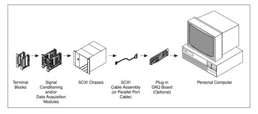
Figure 19-2. Components of an SCXI System
