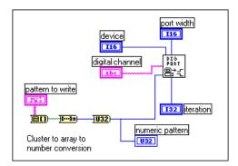
Figure 21-12. Outputting Digital Signals through an SCXI Chassis
