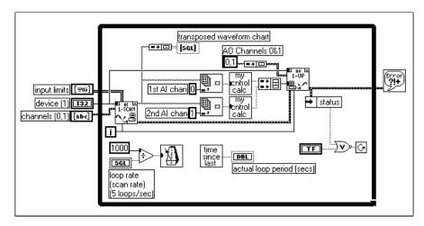
Figure 6-7. Software-Timed Analog I/O
