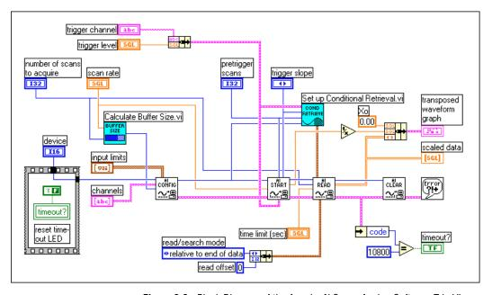
Figure 8-9. Block Diagram of the Acquire N Scans Analog Software Trig VI
