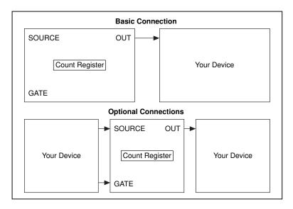
**Figure 24-5.** Physical Connections for Generating a Square Pulse
