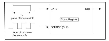
Figure 26-1. Measuring Square Wave Frequency
