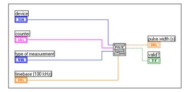
Figure 25-5. Diagram of Measure Pulse Width (9513) VI
