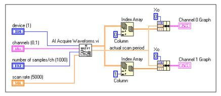
Figure 7-5. Simple Buffered Analog Input Example
