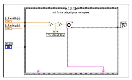
Figure 24-11. Frame 2 of Delayed Pulse (8253) VI
