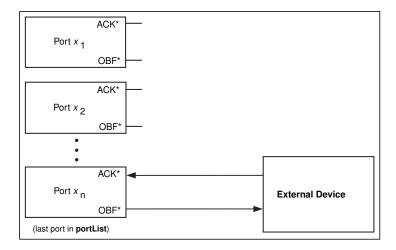
Figure 17-2. Connecting Digital Signal Lines for Digital Output
