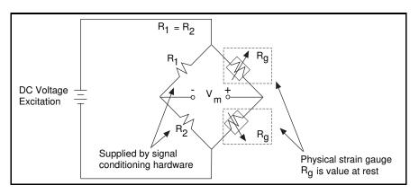
Figure 21-7. Half-Bridge Strain Gauge
