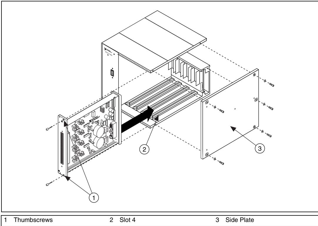
**Figure 3.** Side Plate Removal and Module Installation
