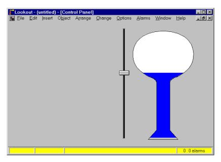
Press <CTRL-SPACE> to toggle out of edit mode and move the slider up and down to see the fill effect created with your tank mask and bar graph. Then get back into edit mode so you can create a trend of the tank level.
