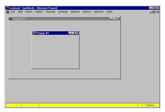
This example displays a **Normal** control panel in a maximized state and two **Popup** control panels in a "popped up" state.
