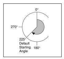
**Rotational sweep** specifies the number of degrees clockwise that the needle will rotate as the **Signal** approaches the **Maximum** value. As shown in the diagram here, you count the **Rotational sweep** in degrees clockwise from the **Starting angle**.
