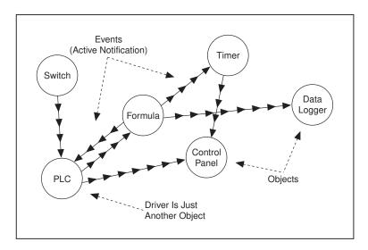
Figure 2-5. Lookout object-oriented and event-driven architecture
