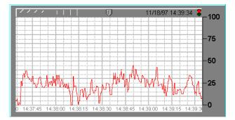
This shows the imaginary scale of the first expression (where min.=0 and max.=100). Because the expression ranges from 0 to 50, it is plotted in the bottom half of the graph.
