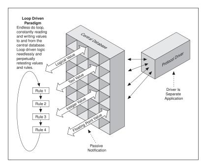
Figure 2-4. Example of conventional, Loop-Driven software program
