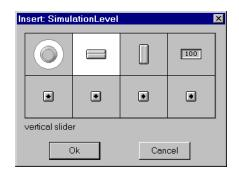
Choose the vertical slider display and select **OK**. Lookout inserts the pot on the active control panel. You can now stretch or reposition the potentiometer anywhere on the panel using the sizing handles.
