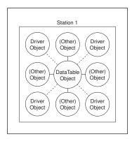
The focus of this picture is the driver objects and their connections to the DataTable. Eventually you will modify this process file to run at Station2 and Station3 by deleting all connections to Driver objects, and then deleting the driver objects themselves at Stations 2 and 3.
