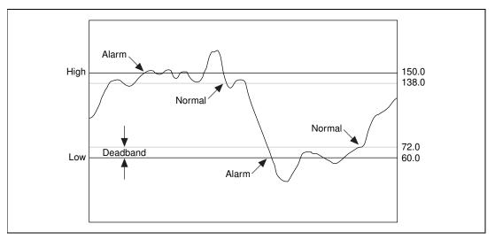
Figure 4-4. Alarm processing of a data member whose alarm setpoints are shown and whose **Deadband** is 12
