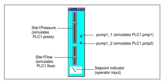
Use two slider pots as your pressure and flow outputs, and two switches as the on/off indicators for pumps one and two. You can use the dial gauge at
