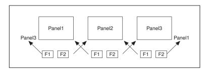
In similar fashion, the F1 data member of Panel3 is connected to the activate data member of Panel2 and the F1 data member of Panel2 is connected to the activate data member of Panel1. So now, Panel2.activate = Panel1.F2 OR Panel3.F1. An operator can depress F2 to page forward through the control panels and F1 to page back through the control panels.
