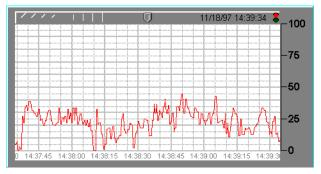
This figure shows the imaginary scale of the first expression (where min.=0 and max.=100). Because the expression ranges from 0 to 50, it is plotted in the bottom half of the graph.
