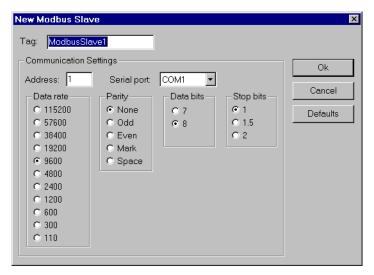
Figure 18-69. Modbus Slave Configuration Parameters Dialog Box
