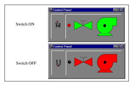
The Switch is shown in both the On and Off positions. The graphics on the right side of the control panel show three ways of graphically displaying the logical signal generated by the Switch.
