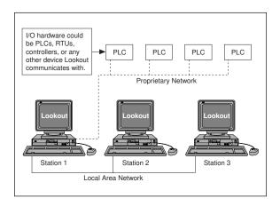
By doing a little planning, you can configure Lookout at Station1 so that you can reuse its process file at Station2 and Station3. The following diagram depicts the general design of the Lookout process file at Station1. Notice that driver objects are connected to the DataTable object using dotted lines while all other objects are connected using solid lines. This is for illustrative purposes only.
