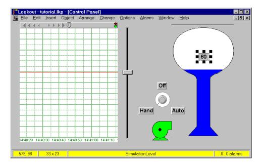
Toggle out of edit mode so you can test your system. Turn the HOA switch to the Auto position and run the slider up and down to see if the Neutralzone is working correctly. Then turn the HOA switch to the Off and Hand positions to complete your testing. The pump should change colors according to your logic.
