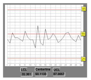
Figure 18-134. X-Bar Chart Showing Upper Control Limit, Center Line, and Lower Control Limits.
