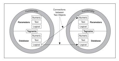
Figure 2-3. Example connections between two objects
