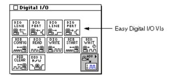
The Easy Digital I/O VIs are the VIs on the top row of the **Digital I/O** palette. For examples of how to use the Easy Digital I/O VIs, open the example library by opening examples\daq\digital\digital.llb.
