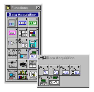
The **Data Acquisition** palette contains six subpalette icons that take you to the different classes of DAQ VIs. The following illustration shows what each of the icons in the **Data Acquisition** palette means.
