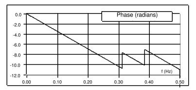
The discontinuities in the phase response arise from the discontinuities introduced when you compute the magnitude response using the absolute value. Notice that the discontinuities in phase are on the order of *pi*. The phase, however, is clearly linear. See Appendix D, *References*, for material that can give you more information on this topic.
