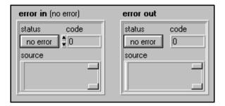
You can find the **error in** and **error out** clusters by selecting **Controls»Array & Cluster** on the front panel.
