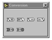
Array Of Strings To Path accepts one-dimensional (1D) arrays of strings, Path To Array Of Strings accepts paths, Path To String accepts paths, and String To Path accepts strings.
