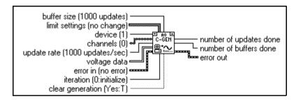
iteration terminal You use the AO Continuous Gen VI when your waveform data resides on disk and is too large to hold in memory, or when you must create your waveform in real time. Place the VI in a While Loop and wire the iteration terminal to the VI **iteration** input.
