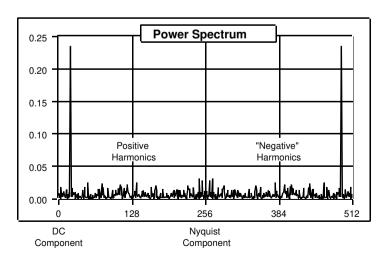
If *n* is odd, let  $k = \frac{n-1}{2}$ . The following table shows the format of the output sequence Sxx corresponding to the power spectrum.
