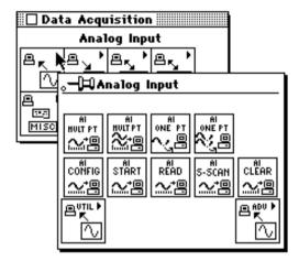
There are four classes of Analog Input VIs found in the **Analog Input** palette. The Easy Analog Input VIs, Intermediate Analog Input VIs, Analog Input Utility VIs, and Advanced Analog Input VIs. The following illustrates these VI classes.
