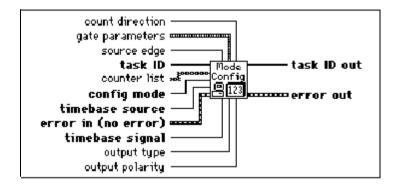
This VI does not start the counters. Use CTR Control VI with **control code** 1 (Start) to start the counters. If you are using a counter for pulse generation, you do not have to call this VI unless you want to change the gate mode or output behavior.
