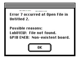
General Error Handler is one of the three error handling utility VIs. It contains a database of error codes and descriptions, from which it creates messages like the previous one. The Simple Error Handler performs the same basic operation but has fewer options. The third VI, Find First Error, creates the error I/O cluster from functions or VIs that output only scalar error codes.
