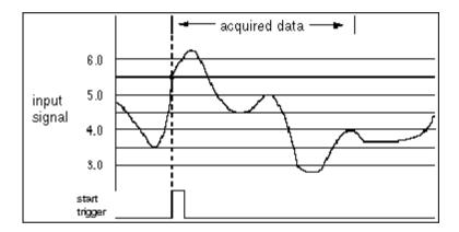
In the above illustration, **total scans to acquire** is 1000 and **pretrigger scans to acquire** is 0. The start trigger can come from digital trigger A or an analog trigger (**trigger or pause condition** =1: Trigger on a rising edge or slope, **level** = 5.5, **window size** = 0.2).
