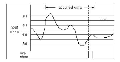
In the above illustration, **total scans to acquire** is 1000 and **pretrigger scans to acquire** is 900. The stop trigger can come from digital trigger A or an analog trigger (**trigger or pause condition** = 1: Trigger on rising edge or slope, **level** = 3.7, **window size** = 0.5).
