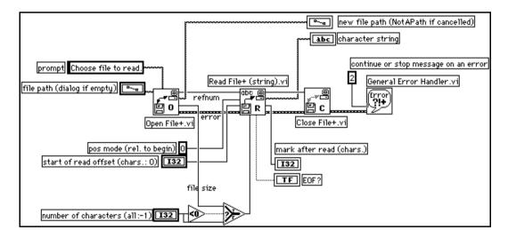
The operation starts at Open File+.vi. If it opens the file successfully, Read File+ (string).vi reads the file and Close File+.vi closes the file. If you pass in an invalid path, Open File+.vi detects the error and passes the error state through the other two VIs to the General Error Handler, which reports it. Notice that the
