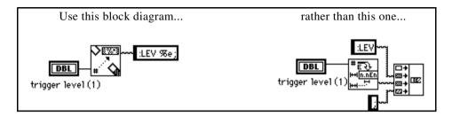
By using Select & Append you can select a string constant and concatenate it to another string in a single step. This procedure is easier than using Select and Concatenate Strings.
