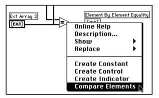
When you compare two arrays of unequal lengths in the **Compare Elements** mode, LabVIEW ignores each element in the larger array
