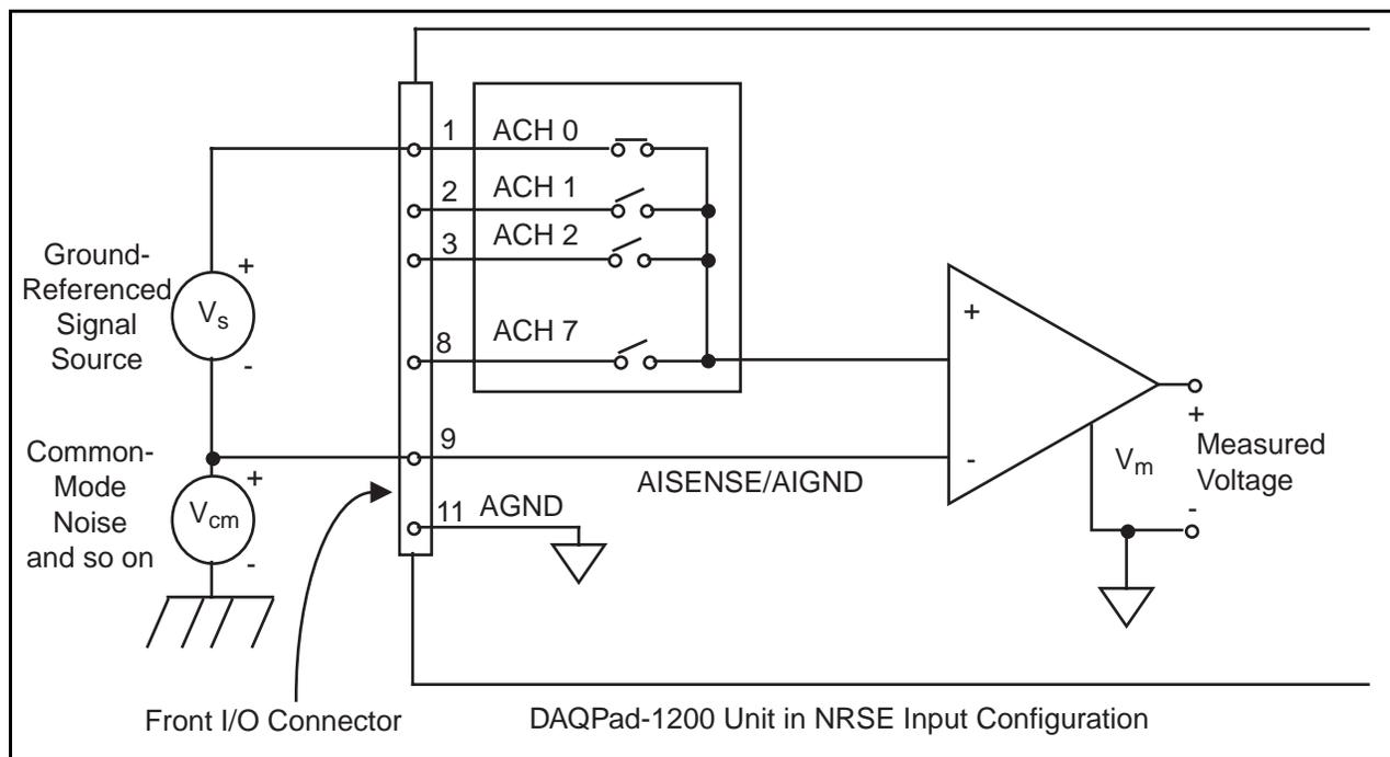
Figure 3-7. Single-Ended Input Connections for Grounded Signal Sources
