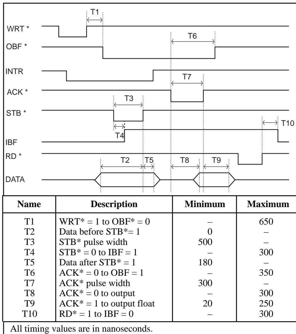
Figure 3-12. Mode 2 Timing Specification for Bidirectional Transfers
