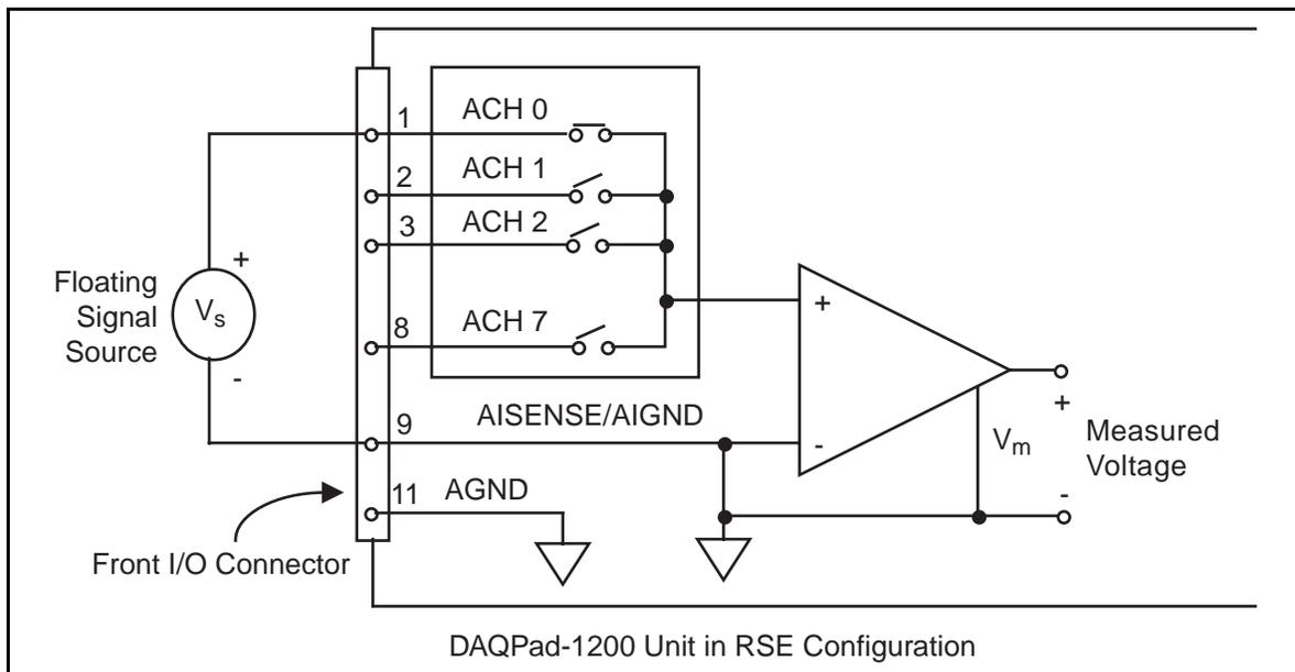
Figure 3-6. Single-Ended Input Connections for Floating Signal Sources
