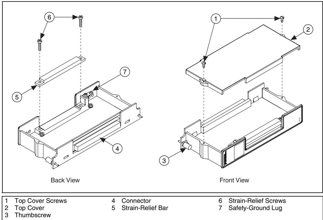
**Figure 3.** SCXI-1317 Enclosure Parts Locator Diagram
