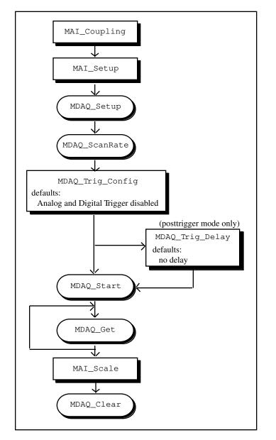
Figure 6-13. Multiple-Channel Data Acquisition with Optional Coupling and Triggering Configuration
