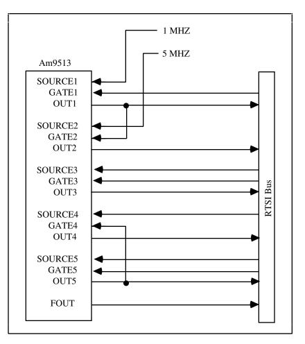
Figure 8-5. NB-DMA-8-G and NB-DMA2800 Counter/Timer Signal Connections
