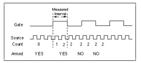
Figure 8-22. Single-Pulse Width Measurement
