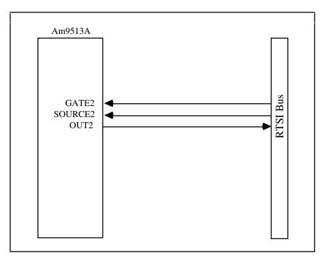
Figure 8-6. NB-A2000 Counter/Timer Signal Connections
