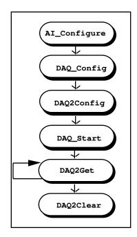
Figure 6-9. Single-Channel, Double-Buffered Acquisition
