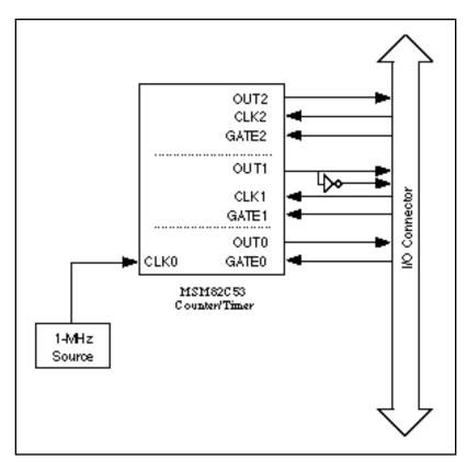
Figure 8-13. DAQCard-500 and DAQCard-700 I/O Counter/Timer Signal Connections
