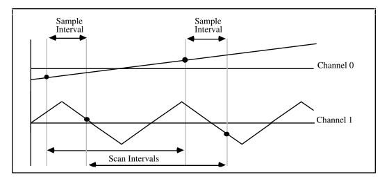
Figure 6-1. NB-MIO-16X Interval Scanning
