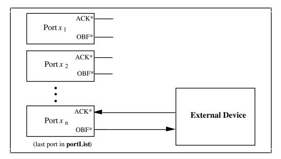
Figure 5-4. Digital Scanning Output Group Handshaking Connections
