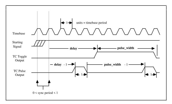
Figure 8-8. Pulse Generation Timing
