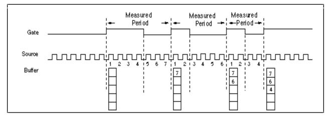
Figure 8-30. Buffered Period Measurement
