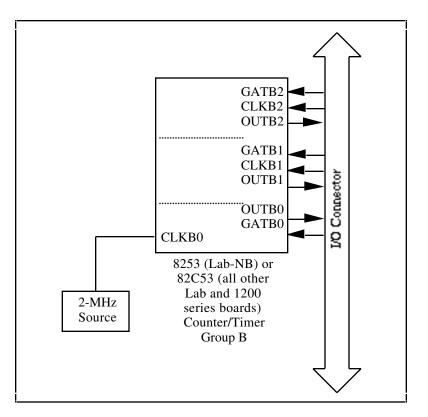
Figure 8-12. Lab and 1200 Series Counter/Timer Signal Connections
