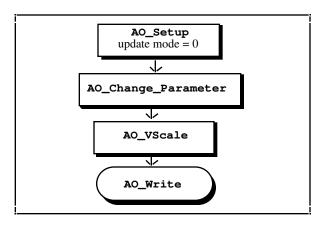
Figure 4-1. Immediate Update Analog Output Flowchart
