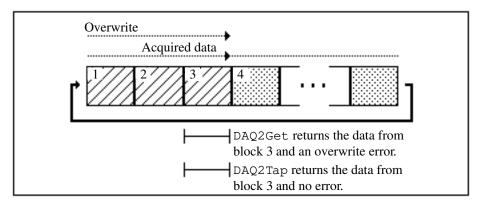
Figure 6-8. Executing DAQ2Get and DAQ2Tap when Overwrite Occurred
