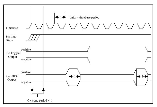
Figure 8-2. Counter Timing and Output Types
