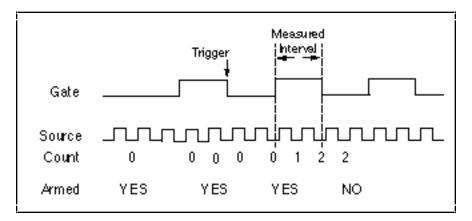
Figure 8-23. Single Triggered Pulse Width Measurement
