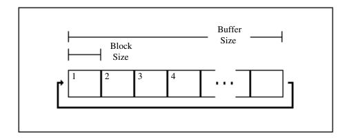
Figure 6-5. Double-Buffered Acquisition Buffer and Blocks
