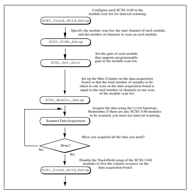
Figure 7-5. Channel-Scanning Operation Using Modules in Multiplexed Mode
