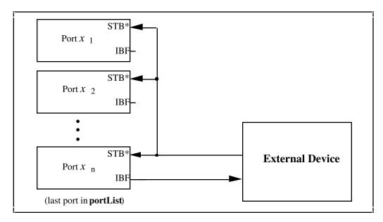
Figure 5-3. Digital Scanning Input Group Handshaking Connections
