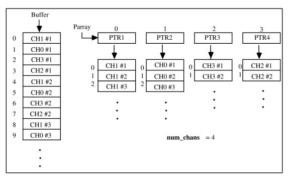
Figure 6-3. SCAN\_Demux Buffer Translation for the Lab and 1200 Series
