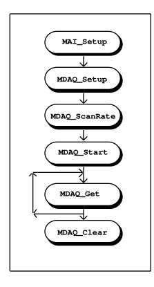
Figure 6-12. Minimum Function Flowchart for Multiple-Channel Data Acquisition
