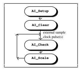
Figure 3-2. Flowchart for Externally Clocked Analog Input Readings
