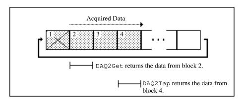
Figure 6-7. Second Execution of DAQ2Get and DAQ2Tap
