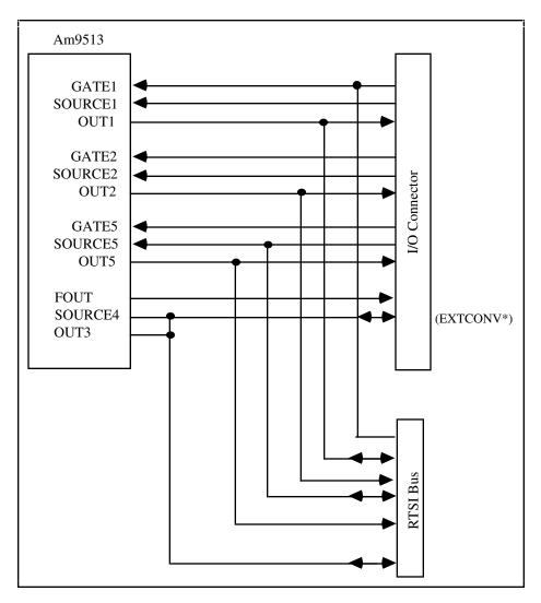
Figure 8-4. NB-MIO-16X Counter/Timer Signal Connections
