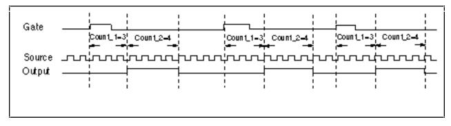
Figure 8-26. Retriggerable Pulse Generation
