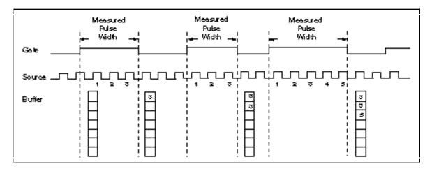
Figure 8-32. Buffered Pulse Width Measurement
