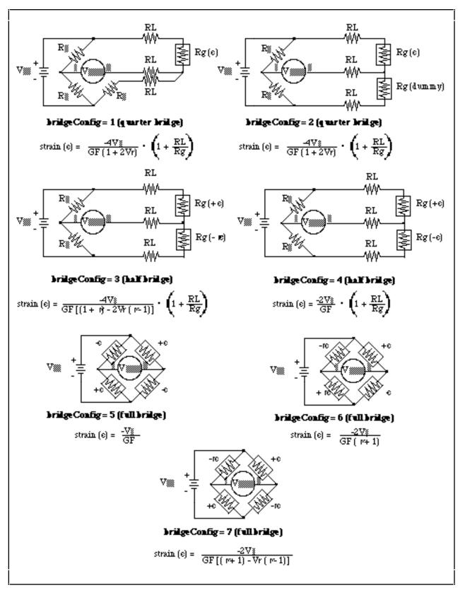
Figure D-1. Strain Gauge Bridge Configurations
