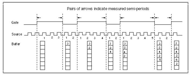
Figure 8-31. Buffered Semi-Period Measurement
