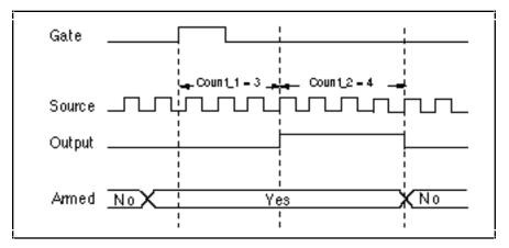
Figure 8-25. Single Triggered Pulse Generation
