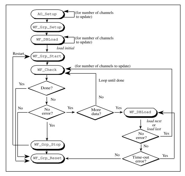
Figure 10-3. Double-Buffered Waveform Generation Flowchart
