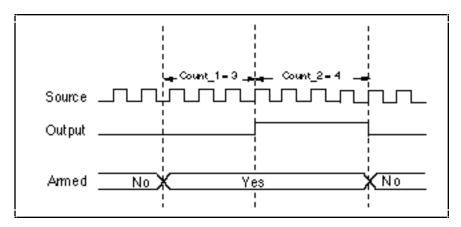
Figure 8-24. Single Pulse Generation
