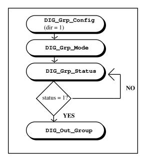
Figure 5-2. Flowchart for Latched Digital Group Output
