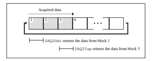
Figure 6-6. First Execution of DAQ2Get and DAQ2Tap
