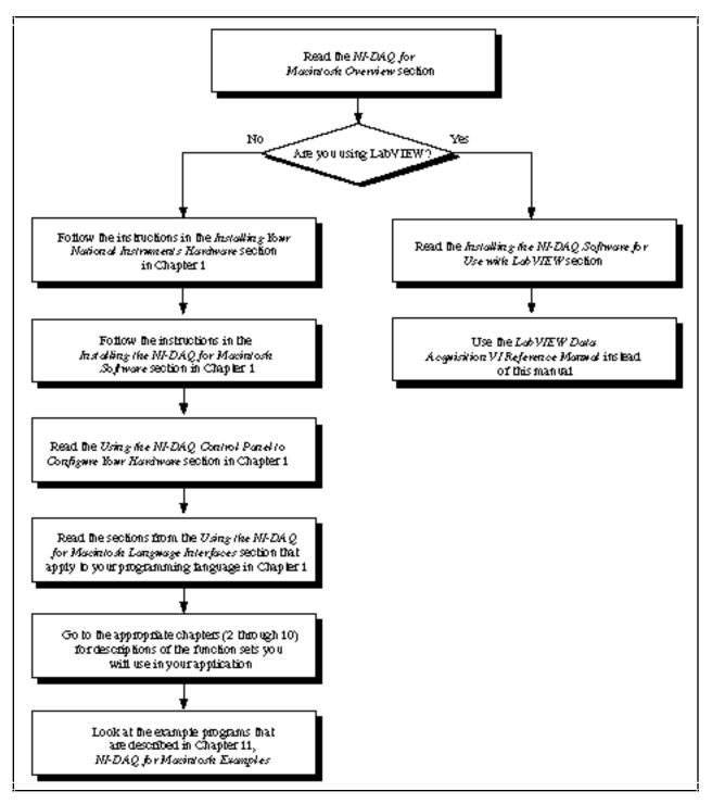
Figure 1-1. Steps to Begin Using NI-DAQ
