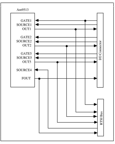
Figure 8-3. NB-MIO-16 Counter/Timer Signal Connections
