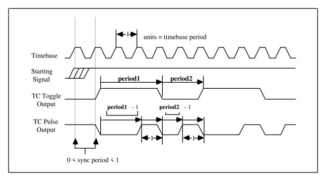
Figure 8-10. Square Wave Timing
