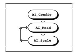
Figure 3-1. Flowchart for Analog Input Readings
