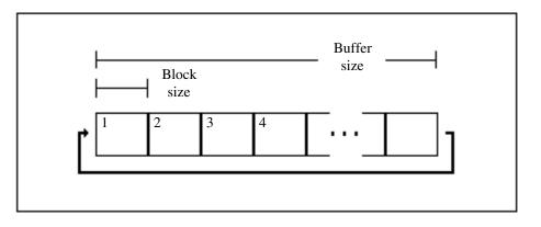
Figure 10-6. Circular Waveform Buffer and Blocks
