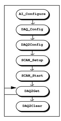
Figure 6-10. Multiple-Channel, Double-Buffered Acquisition (MIO Boards)
