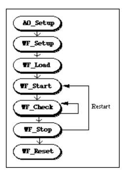
Figure 10-1. Asynchronous Waveform Generation Flowchart
