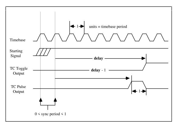
Figure 8-9. Pulse Timing for  $pulse_width = 0$
