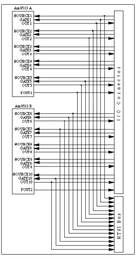
Figure 8-7. NB-TIO-10 Counter/Timer Signal Connections
