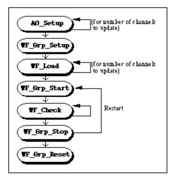
Figure 10-2. Synchronous Waveform Generation Flowchart
