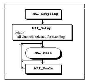
Figure 3-3. Flowchart for Multiple-Channel Analog Input Readings
