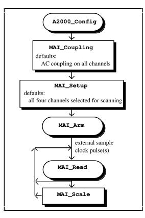
Figure 3-4. Flowchart for Externally Clocked Multiple-Channel Analog Input
