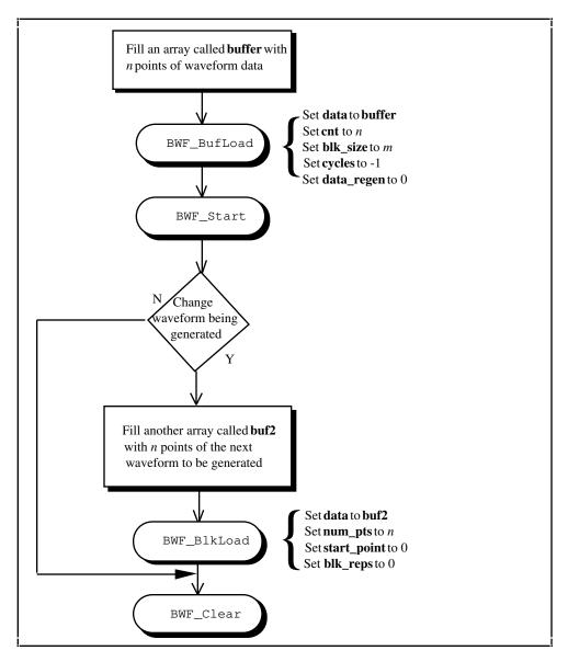
Figure 10-8. Function Generator Application Hints
