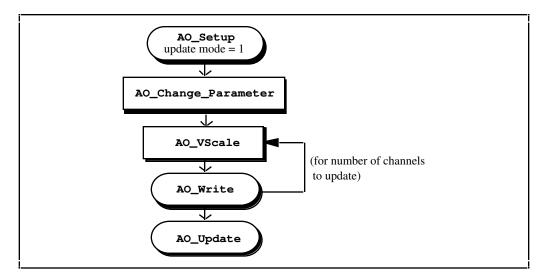
Figure 4-2. Delayed Update Analog Output Flowchart
