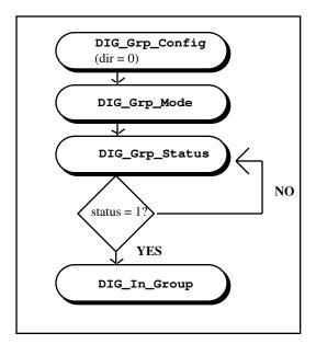
Figure 5-1. Flowchart for Latched Digital Group Input
