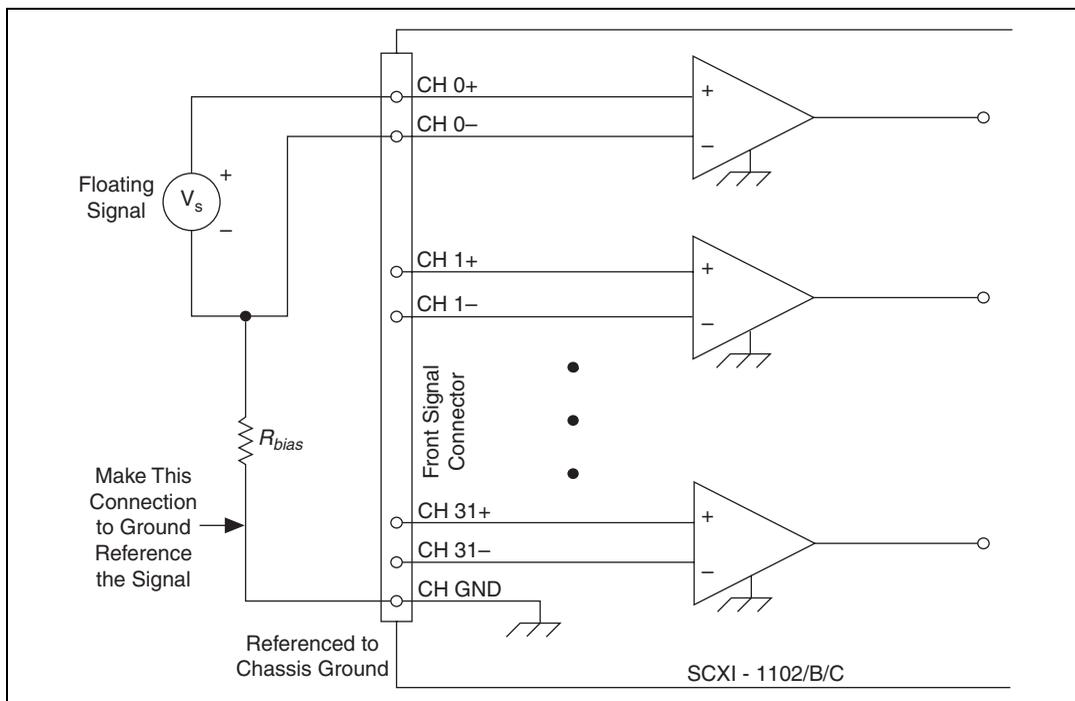
Figure 2-2. Floating Signal Connection Referenced to Chassis Ground
