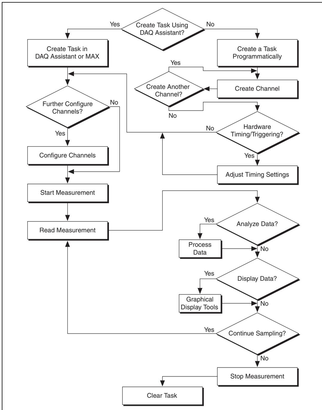
Figure 5-1. Typical Program Flowchart for Voltage Measurement Channels
