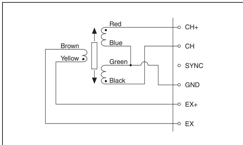
**Figure 2-2.** 5-Wire Connection to an LVDT or RVDT
