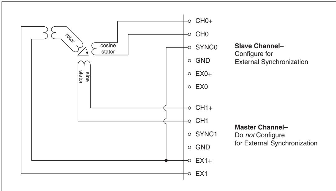
Figure 2-4. Resolver Connection
