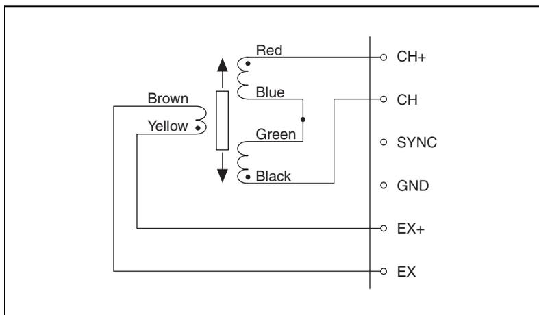
**Figure 2-1.** 4-Wire Connection to an LVDT or RVDT
