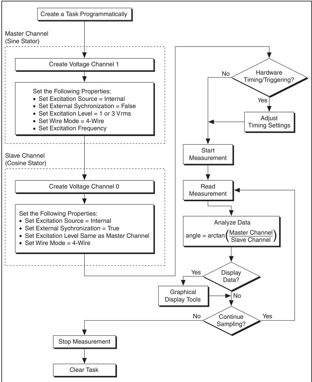
Figure 5-2. Typical Program Flowchart for Resolver Channels
