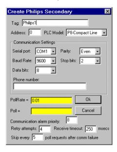
**Serial port** specifies which communications port the object uses for communicating to the external device. This does not specify the communication type. Communication type is determined by the Options—Serial Ports... command.
