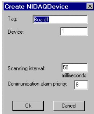
**Device** is the NI-DAQ device number. The DAQ configuration utility (`WDAQConf.exe`) assigns this number to an installed device. Valid device numbers range from 1 to 16.
