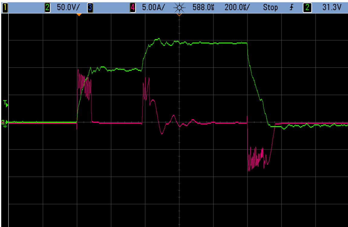
Figure 19b. Current and voltage traces from Piezo IPhaseArray configuration example 5. HVTarget = 150V. Charge voltage = 100V step, then 150V.
