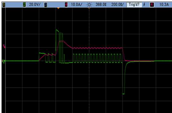
Figure 7. Current and Voltage Traces from Solenoid IPhaseArray Configuration Example 3
