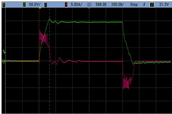
Figure 21. Current and Voltage Traces from Piezo IPhaseArray Configuration Example 2
