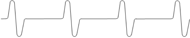
Figure 9. Incorrect Signal Polarity for VR Input Circuit
