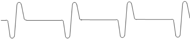
Figure 9. Incorrect Signal Polarity for VR Input Circuit
