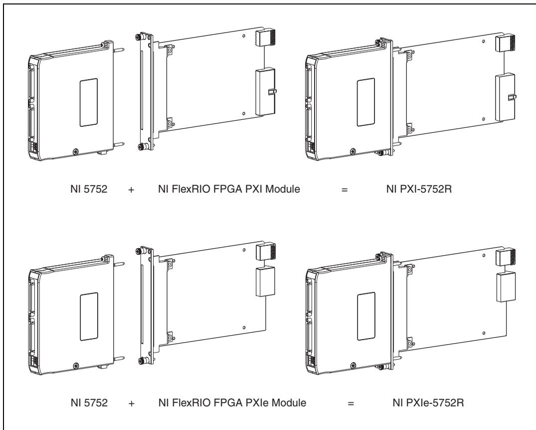
**Figure 1.** FPGA Module and NI 5752 Adapter Module
