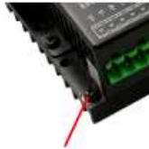
Figure 6. Grounding Screw on the Chassis
