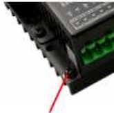
Figure 6. Grounding Screw on the Chassis
