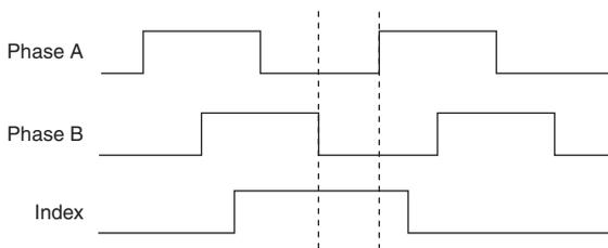
You can set the index reference criteria in software to change the line state of Phase A and Phase B used in the Index search. Refer to the *NI SoftMotion Module* book of the *LabVIEW Help* for more information about encoder settings.
