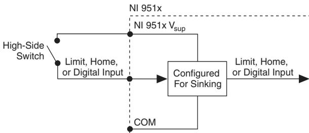
**Figure 3-16.** High-Side Switch Connected to a Sourcing Digital Input
