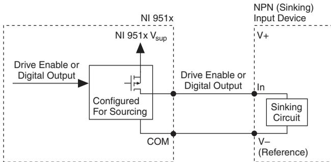
**Figure 3-5.** Drive Enable Circuit Configured for Sinking
