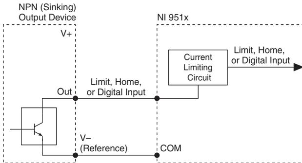
Figure 3-8 shows an example of wiring the inputs to a high-side switch and Figure 3-9 shows an example of wiring the inputs to a low-side switch.
