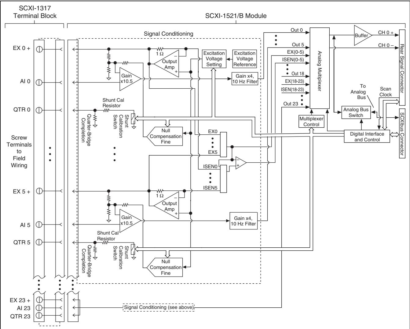
Figure 4-4. Block Diagram of SCXI-1317 and SCXI-1521/B Combination
