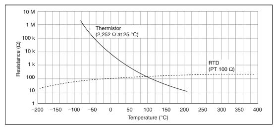
**Figure 4-8.** Resistance-Temperature Curve for a 2,252  $\Omega$  Thermistor
