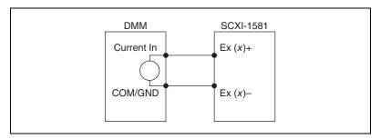
Figure 1-1. SCXI-1581 to DMM Connections
