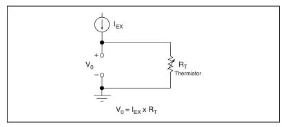
Figure 4-9. Thermistor Measurement with Constant Current Excitation
