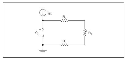
Figure 4-6. 2-Wire RTD Measurement
