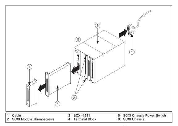
Figure B-1. Removing the SCXI-1581
