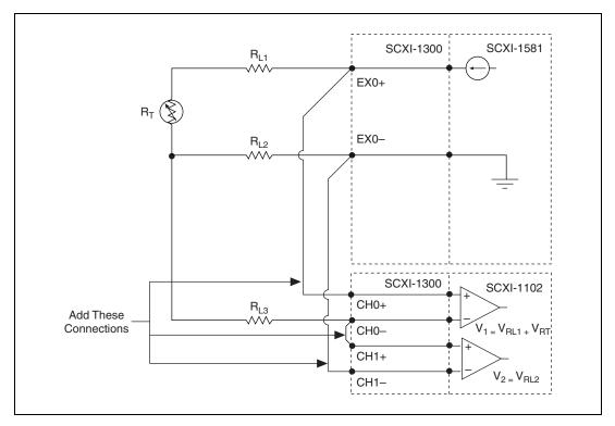
**Figure 4-5.** 3-Wire Configuration Using Two Differential Amplifiers
