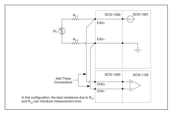
**Figure 4-2.** 2-Wire Resistive Sensor Connected in a 2-Wire Configuration
