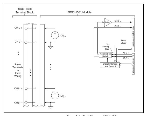
Figure 3-1. Block Diagram of SCXI-1581
