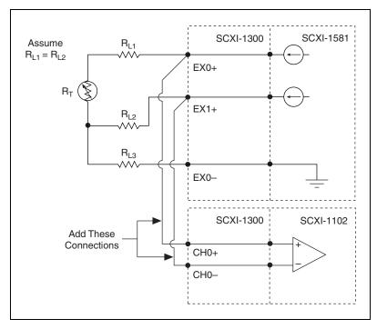
Figure 4-4. 3-Wire Configuration Using Matched Current Sources
