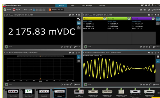
Figure 1. View measurements across USB DAQ, modular and bench instruments all on one BenchVue interface.
