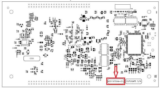
USB-6212 BNC/6216 BNC/6218 BNC – Label can be found on the bottom of the enclosure.
