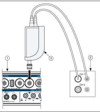
VirtualBench Oscilloscope 2 Oscilloscope Calibrator Oscilloscope Calibrator Active Head
