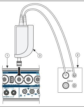
VirtualBench Oscilloscope 2 Oscilloscope Calibrator 3 Oscilloscope Calibrator Active Head
