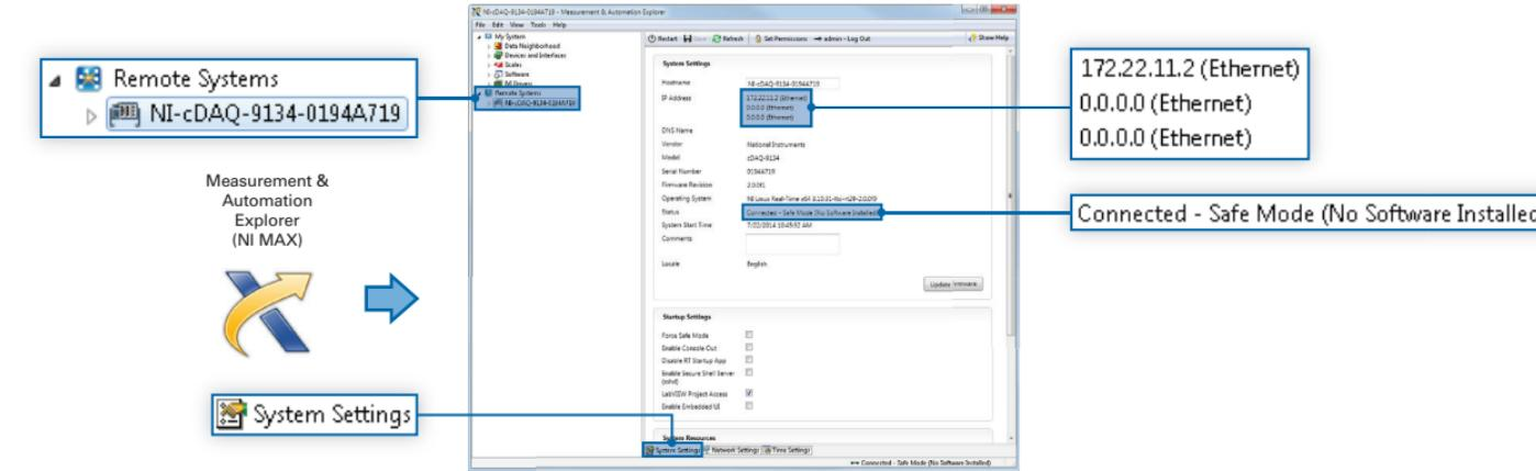
Turn on the external power source. Launch MAX. Expand Remote Systems and select the cDAQ controller. On the System Settings tab, verify that the controller has an IP address and the System State reads **Connected - Safe Mode (No Software Installed)**.
