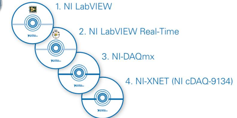
On the host computer, install LabVIEW, LabVIEW Real-Time, and NI-DAQmx. Install NI-XNET last if you are setting up the cDAQ-9134.
