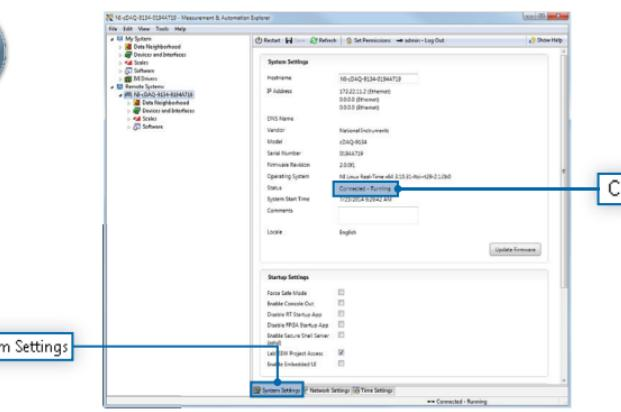
expand Remote Systems and select the cDAQ controller. On the System Settings tab, verify that the System State reads **Connected - Running**.
