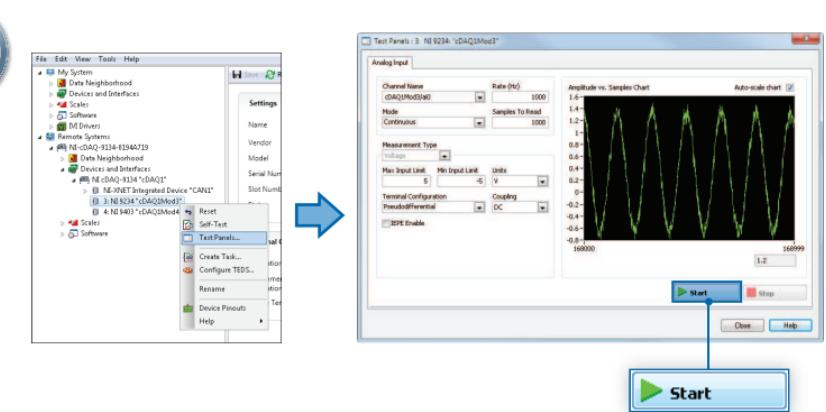
Take your first measurement in MAX. Right-click any module and select **Test Panels**. Configure the measurement settings and click **Start**.
