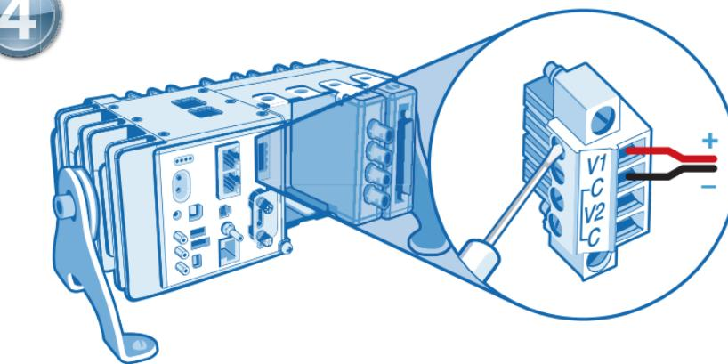
Connect the positive lead of the power source to the V1 terminal on the power connector plug, and the negative lead to one of the C terminals.
