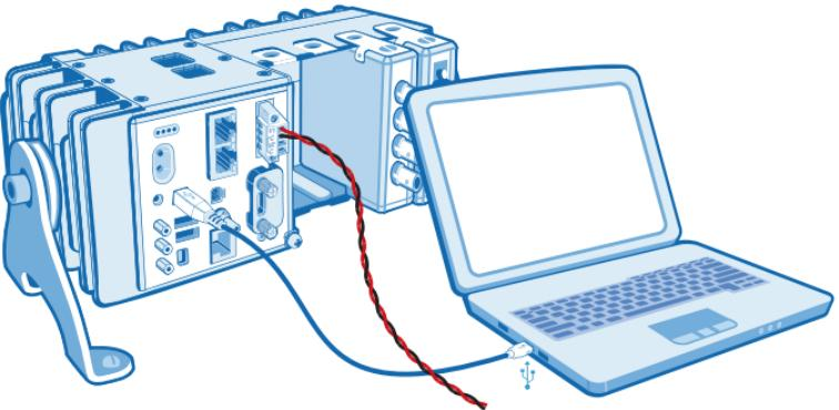
Use the supplied USB A-to-B cable to connect the host computer to the USB device port on the cDAQ controller.
