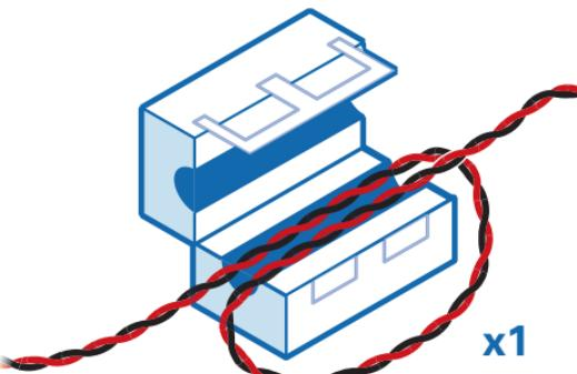
Verify power source is turned off. Install ferrite across the negative and positive leads of the power source.
