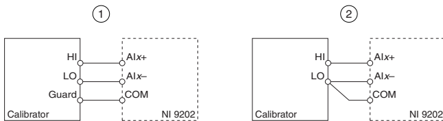
Figure 1. Analog Input Verification Connections
