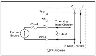
Figure 7. Current Input without an External Power Supply
