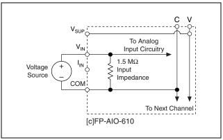
Figure 5. Voltage Input without an External Power Supply
