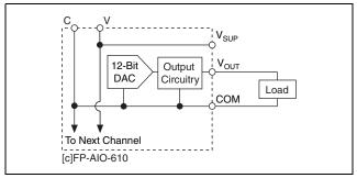
Figure 9. [c]FP-AIO-610 Analog Output Circuit
