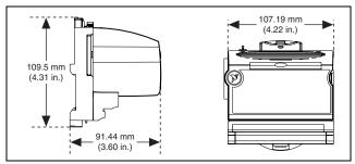
Figure 10. FP-AIO-610 Mechanical Dimensions
