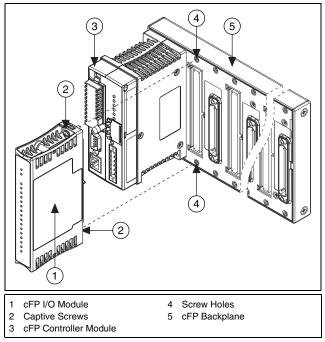
Figure 2. Installing the cFP-AIO-610
