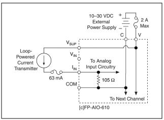
Figure 8. Current Input with an External Power Supply
