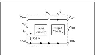
Figure 3. Basic Field Connection
