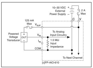
Figure 6. Voltage Input with an External Power Supply
