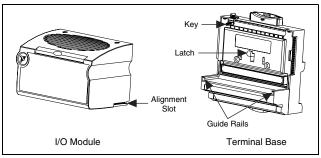
Figure 1. Installing the FP-AO-210
