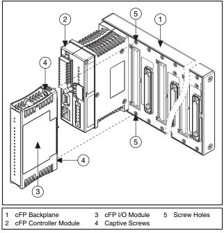
Figure 2. Installing the cFP-AO-210
