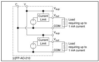
Figure 3. Two Loads without External Supply
