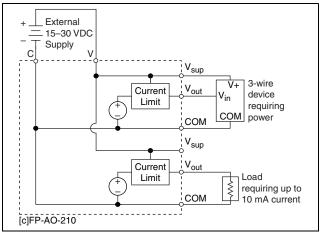
Figure 4. Two Loads with External Supply
