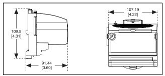
Figure 6. FP-AO-210 Mechanical Dimensions
