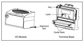
Figure 1. Installing the FP-DO-400
