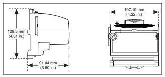
Figure 6. FP-DO-400 Mechanical Dimensions
