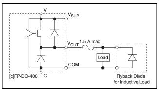
Figure 4. Digital Output Circuit (External Power Supply Not Shown)
