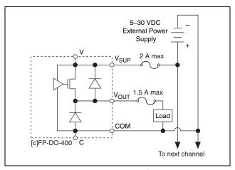
Figure 3. Recommended Field Connections
