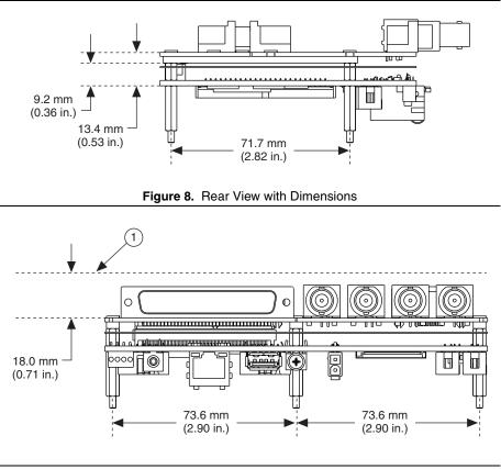
Figure 7. Side View with Dimensions
