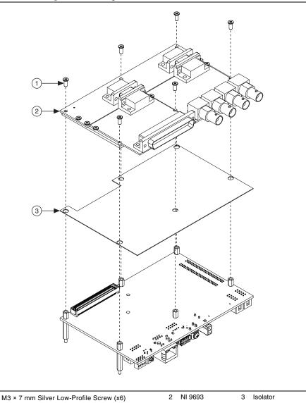
Figure 6. Inserting the Standoffs into the sbRIO Device
